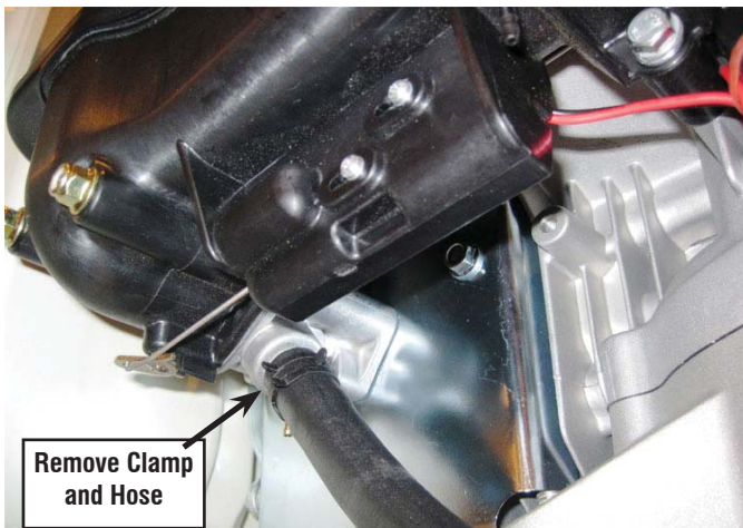
Figure 1.4 — Remove Hose Clamp & Hose
